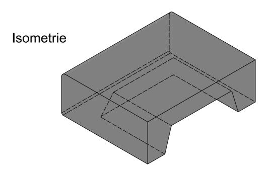
l/b/h/\*) Abweichung je nach Schalungsgeneration: I = 80-100mm; b = 60-100mm; h = 70-80mm; \* = Restmass
